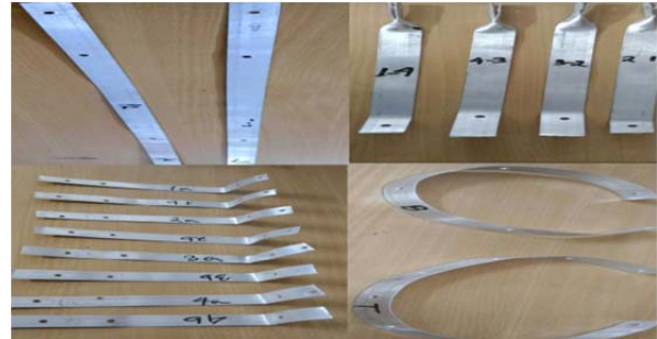
Fig. 9: Different aluminum parts
